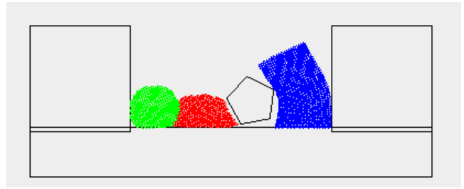
Figure 3: Example of Elastic Particles reacting to the force and pressure exerted upon them by a rigid body
