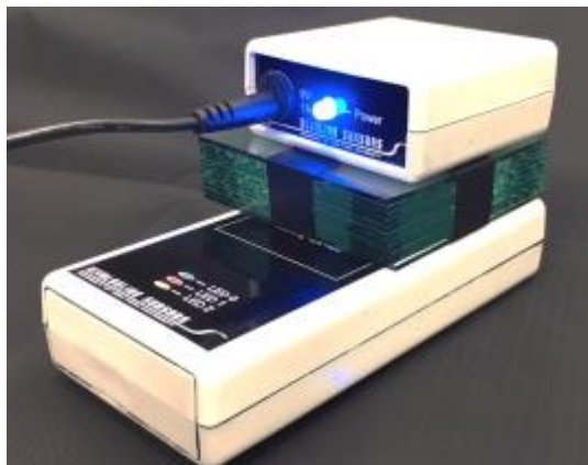
Figure 2. Citygram window-sensor solution showing outside-mic module (bottom), 25mm window glass (middle), and powered inside module (top),
