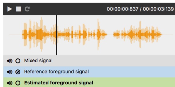
Figure 1: Example of a basic trackswitch.js instance with 3 tracks, a visualization of the waveform, and a seekhead indicating the current playback position.
