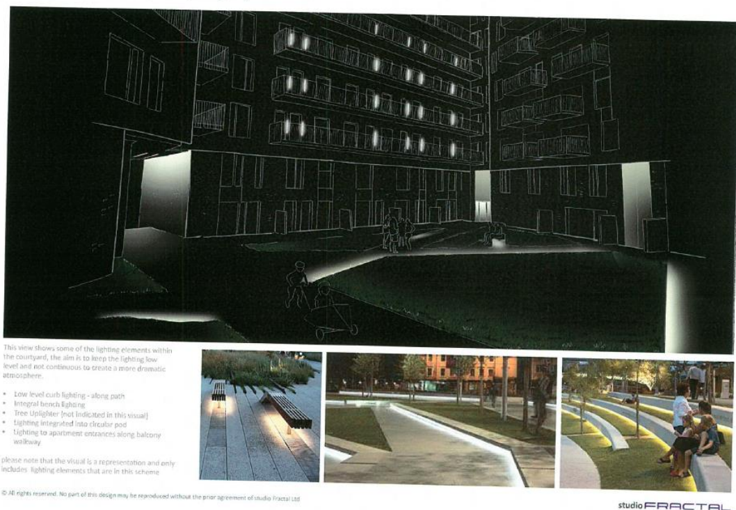
Figure 15: Lighting plan for Phase 3, with lighting embedded in benches and precast concrete curbs in private garden. Source: (Studio Fractal, 2012)
