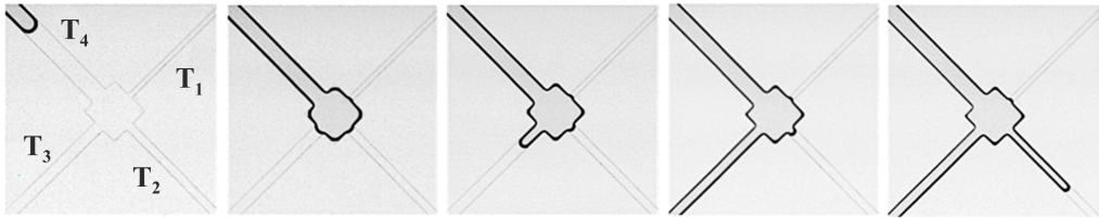
FIGURE 3. Quasi-static primary drainage images in a micro-model (Geometry 2) with etch depth d = 45\mu\text{m} and throat widths w_t : 33, 51, 65, 107\mu\text{m} (WP-white, NWP-grey). Contact angle 26^\circ .
