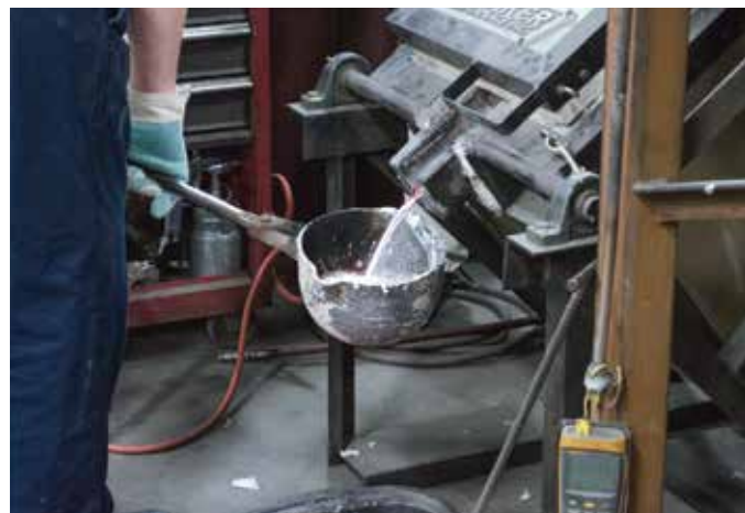
An ORNL scientist pours a new aluminum–cerium alloy from a furnace into a ladle for casting.
