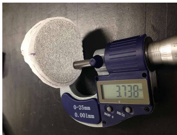
Figure 6.9: For measuring thickness, a digital handheld micrometer was used. The probe has a diameter of 5 mm.
