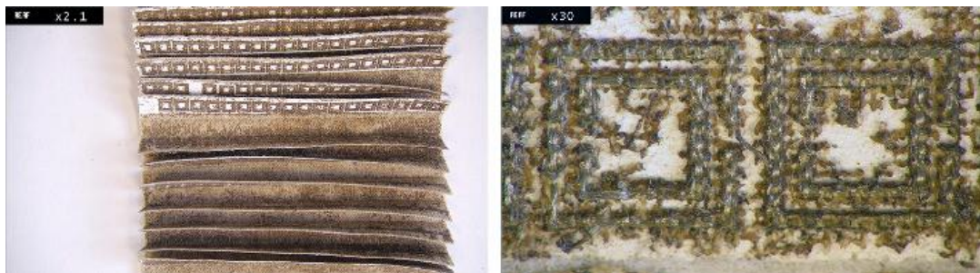
Figure 8.25: Laser-engraved silver cotton. Assembled prototype (left), detail (right).
