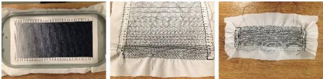
Figure 7.16: Smocking process of Sample 3.
