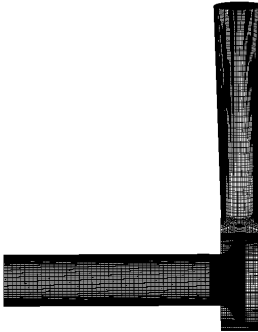
Figure 5.12. Centrifugal pump mesh assembly. Number of elements: 3.14 million
