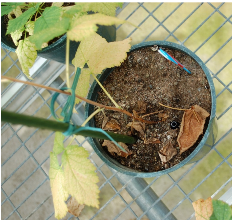
Figure 2.2: A R. idaeus cane with an automated thermal desorption tube in the soil for the passive collection of root volatiles.
