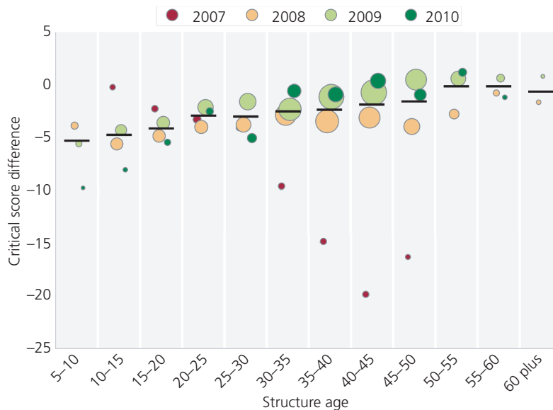
Figure 7. Deterioration rate plots showing the change in BCI_{crit} between successive inspections for populations of structures that were inspected in the same year, split by structure age. The change of condition with time of these populations of bridges has been plotted as the difference between the average BCI scores for the population in each of the successive inspections, weighted by deck area to account for the relative importance of larger structures. The markers have been shaded to indicate the comparison year. The size of the marker has been scaled by the number of bridges that it represents. The weighted average of the plotted comparison years has been plotted on the top as a black bar. Data from 2397 bridges are included in this plot
