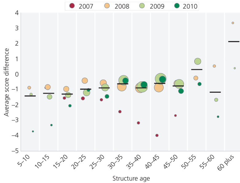
Figure 6. Deterioration rate plots showing the change in BCI_{ave} between successive inspections for populations of structures that were inspected in the same year, split by structure age. The change of condition with time of these populations of bridges has been plotted as the difference between the average BCI scores for the population in each of the successive inspections, weighted by deck area to account for the relative importance of larger structures. The markers have been shaded to indicate the comparison year. The size of the marker has been scaled by the number of bridges that it represents. The weighted average of the plotted comparison years has been plotted on the top as a black bar. Data from 2397 bridges are included in this plot
