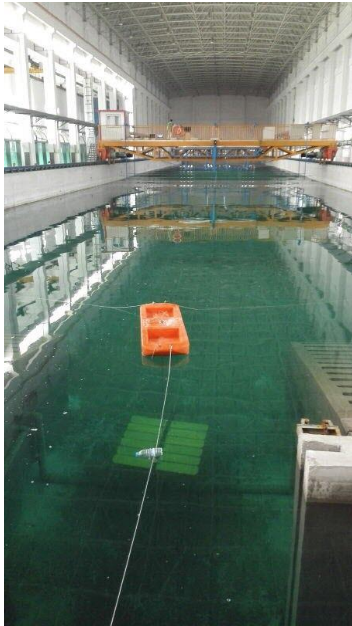
Fig.5. Free sailing test of the wave glider in waves
