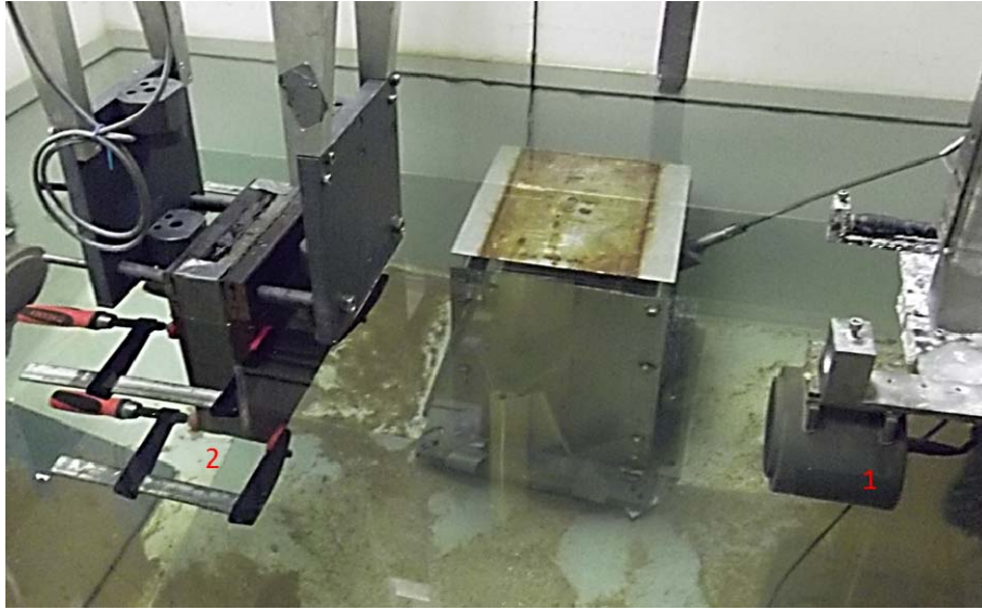
Figure 8. Experimental set-up showing the ultrasound transmitter-receiver (1) and the steel-concrete-steel-sample (2), which is clamped to maintain contact between the concrete and the free steel plate.
