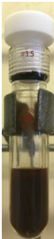
Figure S17: A typical lignin reaction in a glass tube reactor showing the solubility of lignin in acetonitrile.
