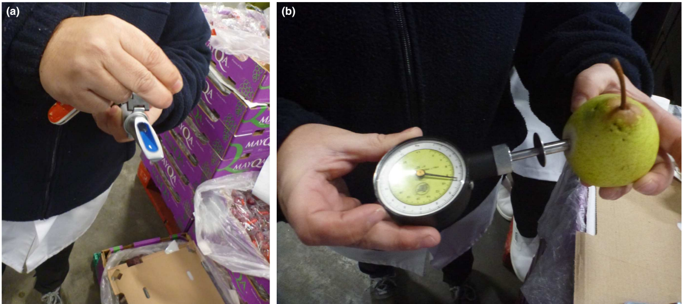
FIGURE 3 Use of refractometer and penetrometer to assess qualities of food (photographs taken by the authors).
