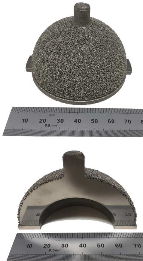
Fig. 2. The geometry of the examined AM acetabular hip prosthesis cup is hemispherical and the lattice structure that ensures optimum bone ingrowth is non-unidormal.
