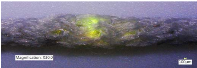
Fig. 1. An E-yarn containing an LED, shown at 30 x magnification
