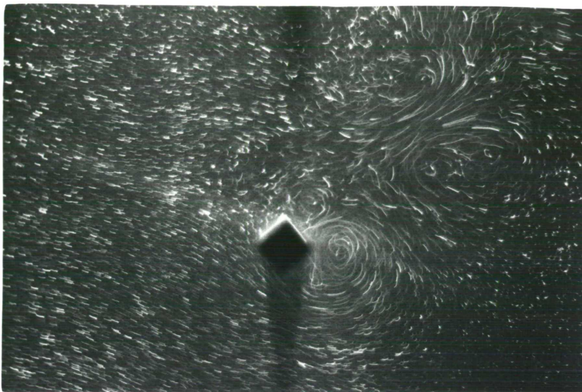
FIG: 5-10(a). Sideways Vortex Street. NKC = 13.61 : t/T \approx 0.68
