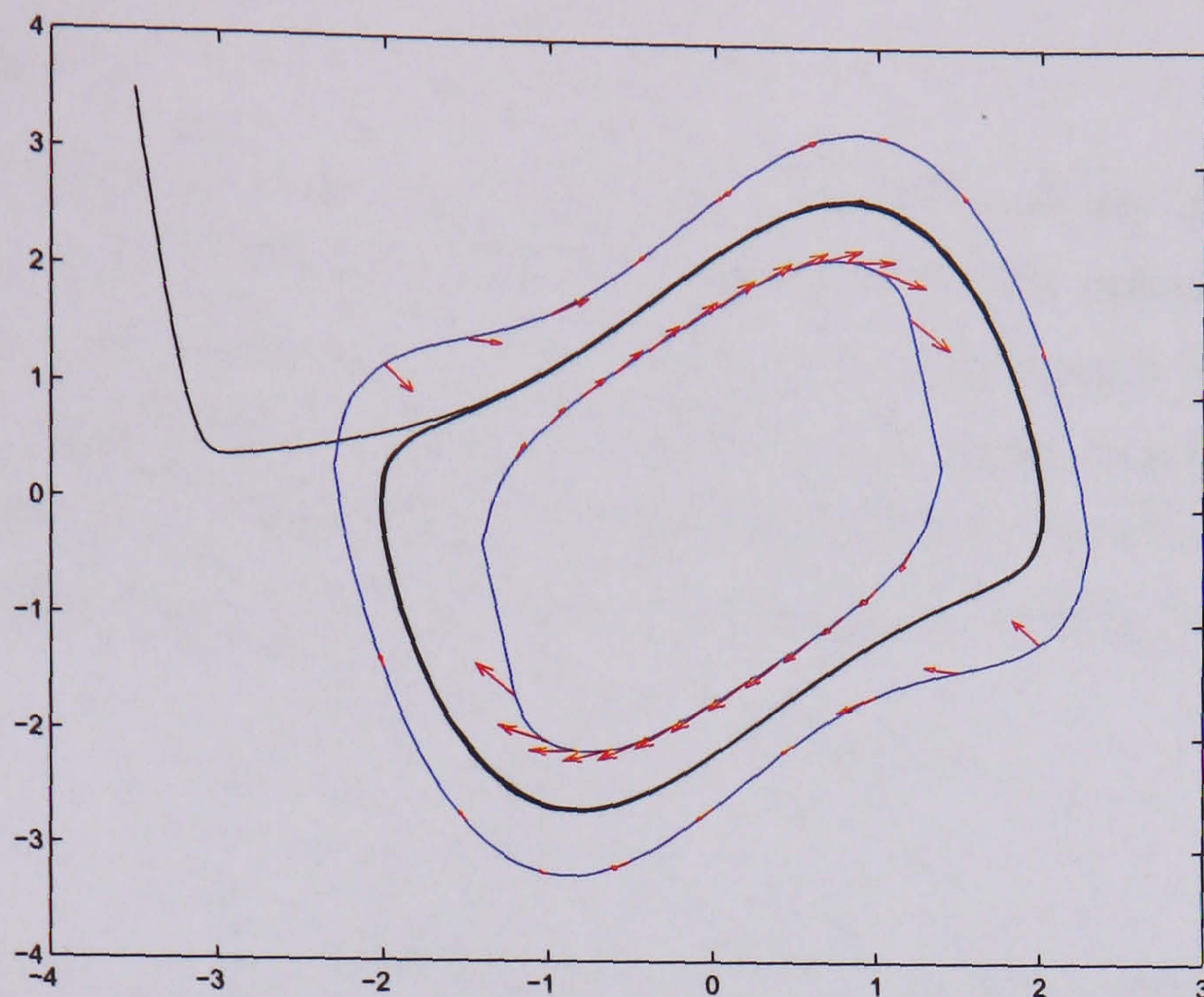
Figure 4.3: Solution trajectory of the van der Pol oscillator in \mathcal{B} . The boundaries of the positively invariant set \mathcal{B} are given in blue; the gradient field on these is indicated by vectors (red); and the trajectory of the van der Pol Oscillator is in black.
