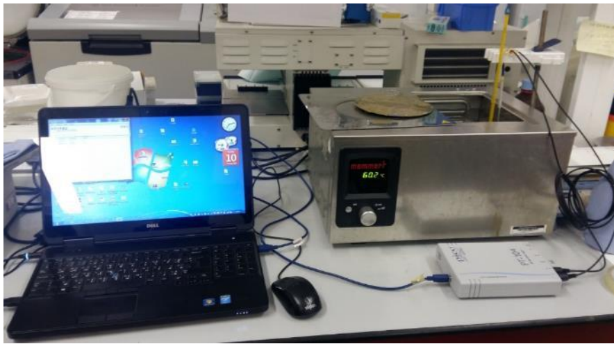
Figure A.1 RTD Sensors Calibration Equipment
