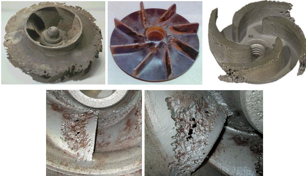
Figure 1-14: Cavitation damage in centrifugal pump impellers [31, 32]
