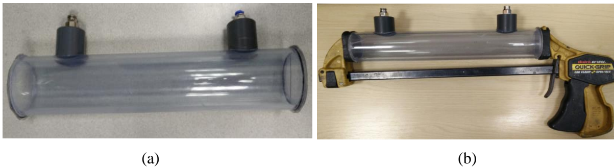
Figure 4-18: (a) Calibration pipe, and (b) Clamp to prevent a possible failure in the pipe
