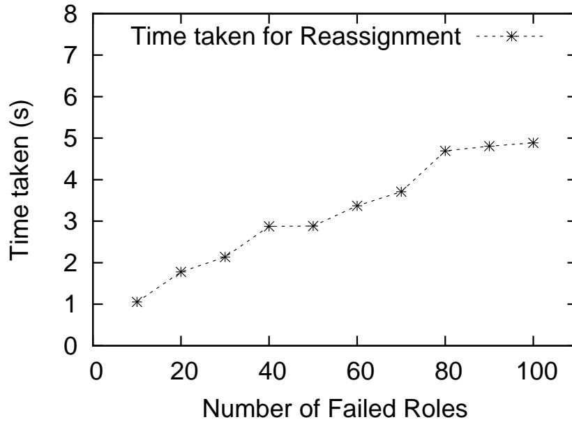
Figure 8.7: Measurement of Time Taken to Reassign Roles in a Cluster Failure Scenario
