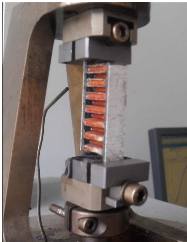
Figure 3: Configuration of a segment of the core shear deformation in the TMA device
