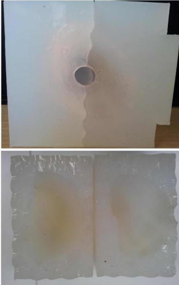
Figure 4.8: Two-part silicone rubber mould.
