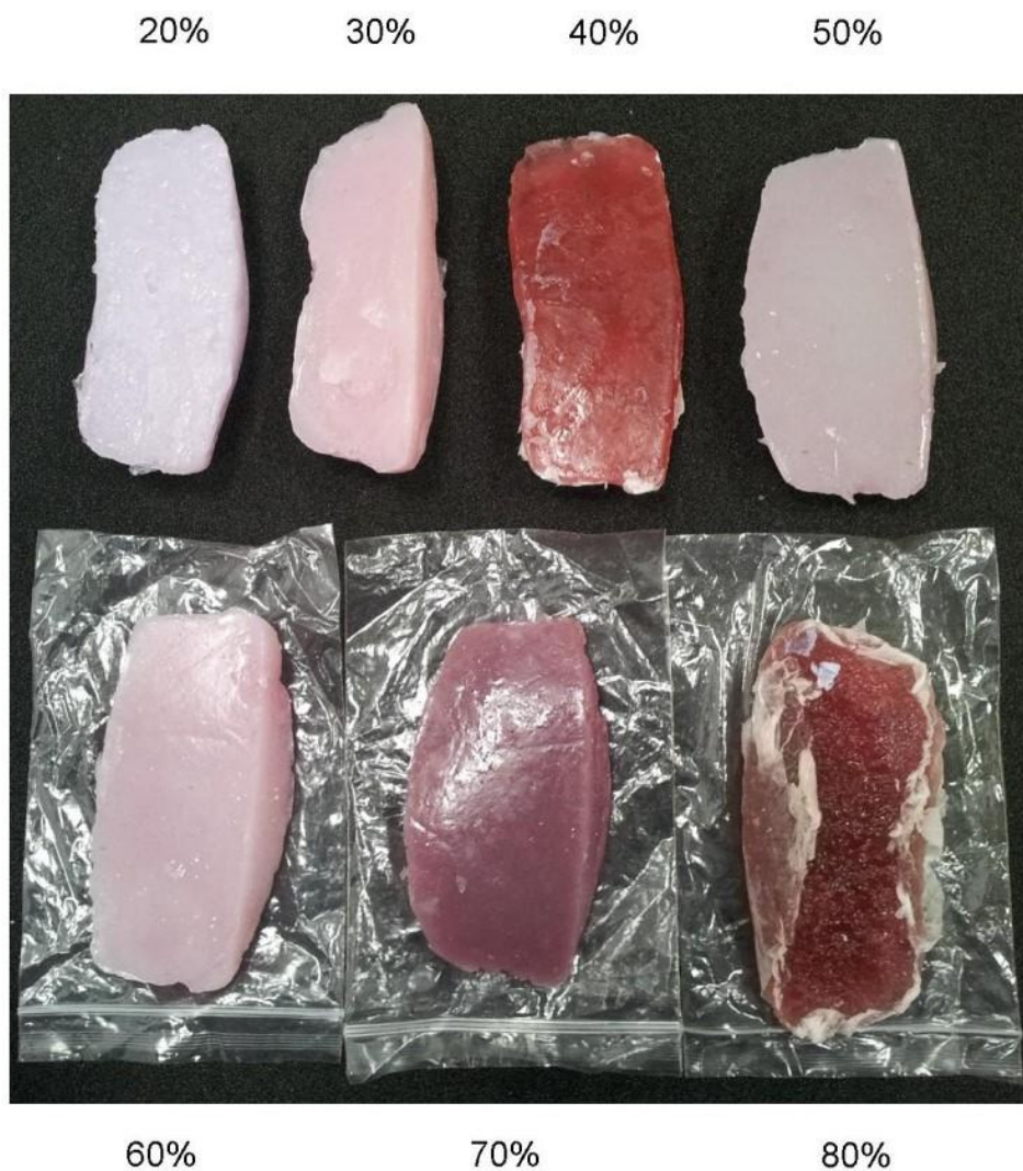
Figure 7.1: Human kidney simulants. The percentage values refer to the Pro Gel 10 softener concentration (% v/v) in each case.
