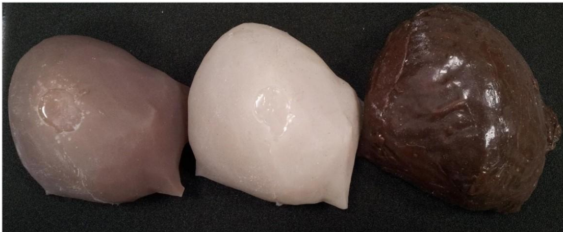
Figure 7.3: Human liver simulants. The percentage values refer to the Pro Gel 10 softener concentration (% v/v) in each case.
