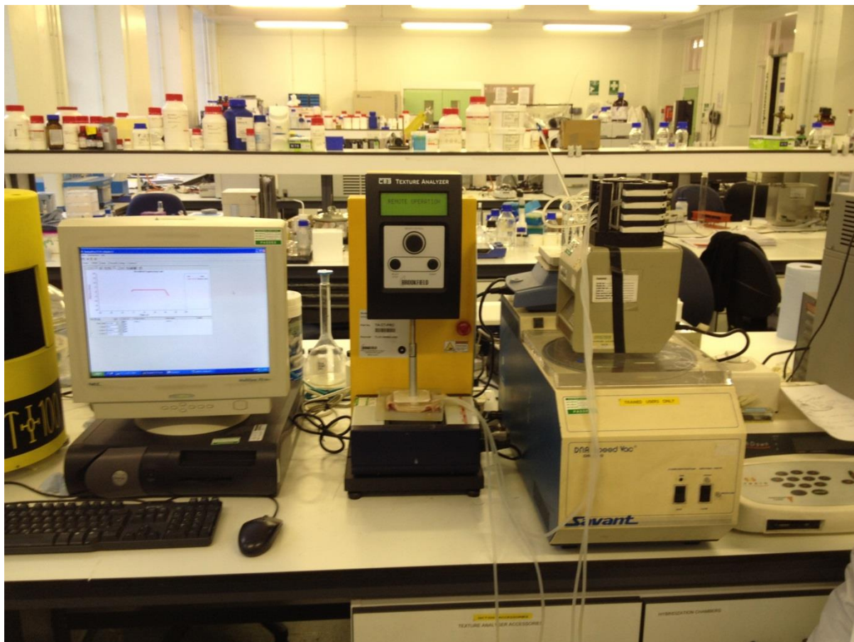
Figure 6.4: An image of Phase One of the modified disintegration test being developed. It shows the texture analyser probe using a large upper palate pressing down on to an ODT which is placed upon the bovine tongue. The heating block maintains tongue temperature at 37 °C, and a hot plate placed behind the peristaltic pump is used to keep saliva at 37 °C.
