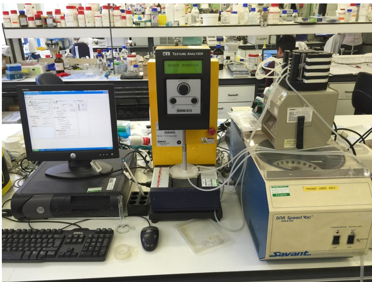
Figure 6.5: An image of Phase Two of the modified disintegration test being developed. It shows the texture analyser probe with an ODT attached by double sided sticky tape. The disintegration bed is a watch glass with 10 ml of water with a piece of filter paper placed on top to simulate the tongue. The heating block maintains temperature at 37 °C, and a hot plate placed behind the peristaltic pump is used to keep saliva at 37 °C.
