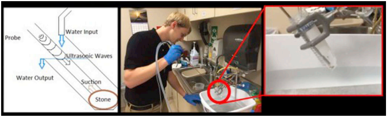
Figure 2. our ex-vivo experiment to measure time to comminution for each stone
