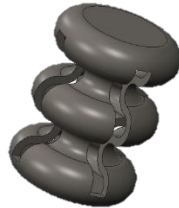
Figure 5: Rubber spring to be used as a connection among compliant mechanisms.
