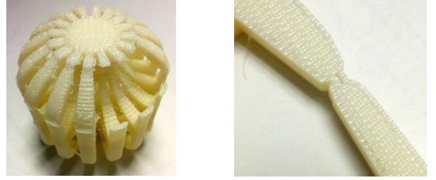
Figure 3: 3D-printed topology in ABS. The picture on the left shows the design of a 3D cellular compliant mechanism with multiple output port radial directions. The picture on the right shows the compliant mechanism hinge in detail.
