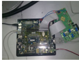
Toradex board with CAN interface and Colibri PXA270 connected to AER-Robot board.
