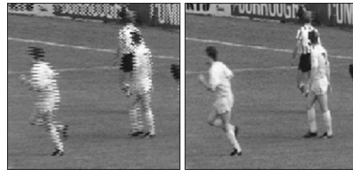
Fig. 8. If picture-repetition is assumed incorrectly, feathering (left) will show.
