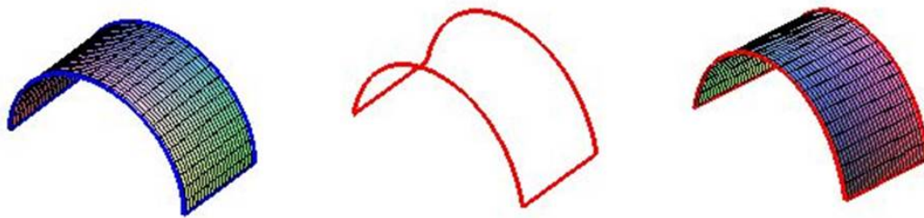
Figure 5: Approximation of a piece of circular cylinder.
