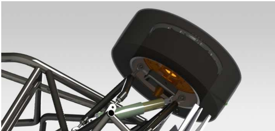
Figure 6.11: Front suspension (model for Simmechanics).
