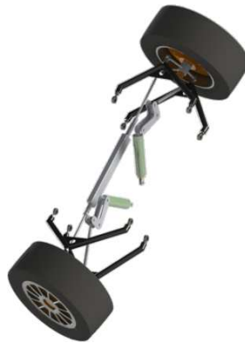
Figure 6.10: Steering system (model for ADAMS).
