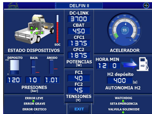
Figure 2.15: Main display of the HMI.
