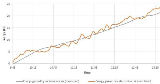
Figure 4.14: 6/21/2013 test energy gain in the cabin air.
