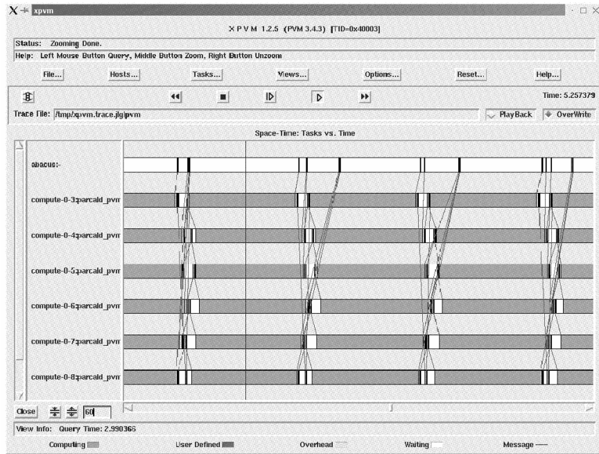
Fig. 9 Gantt chart depicting a detail of the tasks executed by each cluster node and the messages transferred between different nodes versus time. The exchange of neighboring states between nodes processing adjacent partitions at the beginning of each iteration acts as a synchronization point.
