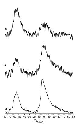
Figure 8.  $^{27}$ Al MAS NMR spectra of the: a)  $V_{Na}$ , b)  $V_{Na~600C}$ , and, c)  $V_{Na~300s}$  samples.
