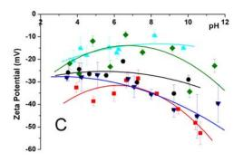
Figure 4: Zeta potential curves (A) raw; (B) thermally treated and (C) mechanically treated samples. Symbols indicate: ( $\triangle$ )  $V_{AI}$ ; ( $\bullet$ )  $V_{Ca}$ ; ( $\bullet$ )  $V_{K}$ ; ( $\blacksquare$ )  $V_{Li}$  and ( $\blacktriangledown$ )  $V_{Na}$  samples.
