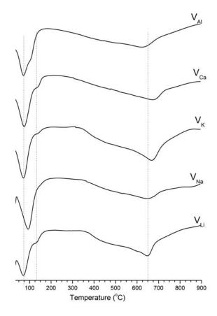
Figure 5. DTA curves of the raw samples
