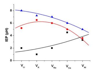
Figure 3: IEP for (■) raw; (●) thermally and (▲) mechanically treated samples (data extracted from [5])
