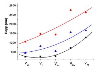
**Figure 1**: Dapp values of indicated samples in: (■) aqueous and ionic strength suspensions (▲) 10<sup>-2</sup> M MCI (chloride of the respective cations) and (●)10<sup>-3</sup> M KCI.
