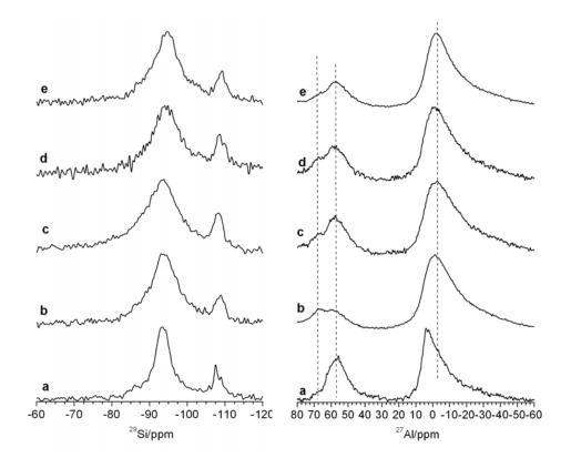
**Figure 7.** <sup>29</sup>Si and <sup>27</sup>Al MAS NMR spectra of the a)  $V_{Na}$ , b)  $V_{Li}$ , c)  $V_K$ , d)  $V_{Ca}$ , and e)  $V_{Al}$  samples
