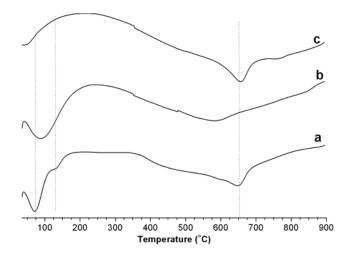
**Figure 6.** DTA curves of the a) V<sub>Li</sub>, b) V<sub>Li 300s</sub> and, c) V<sub>Li 600C</sub> samples.
