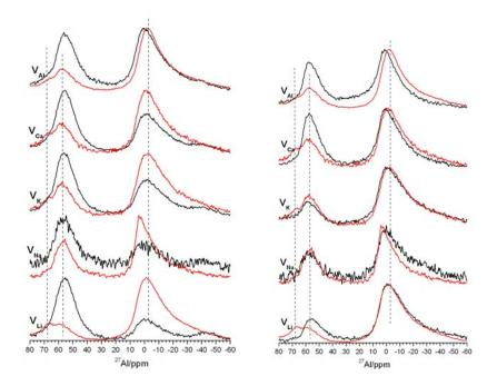
**Figure 9**. <sup>27</sup>Al MAS NMR spectra of montmorillonite: raw (red) mechanically treated (left, black) and heated at 600°C (right, black).
