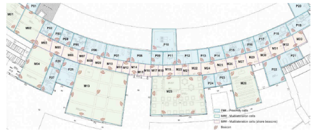
Fig. 2. Beacon deployment in the service floor of the residence. P## are proximity cells, with only one or two beacons, and M## are multilateration cells, with enough beacons to perform multilateration. The areas covered by P-cells and M-cells are 800 and 1200 m 2 respectively.
