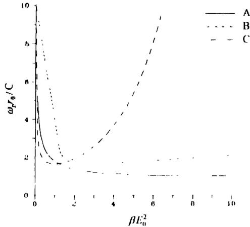
**Figure 6.** Dependence of normalised beam radius ( $\omega_p r_0/c$ ) on incident beam intensity parameter ( $\beta E_0^2$ ). Curve A for present analysis, Curve B for variational method and Curve C for paraxial ray method  $r_0 = 30 \mu\text{m}$
