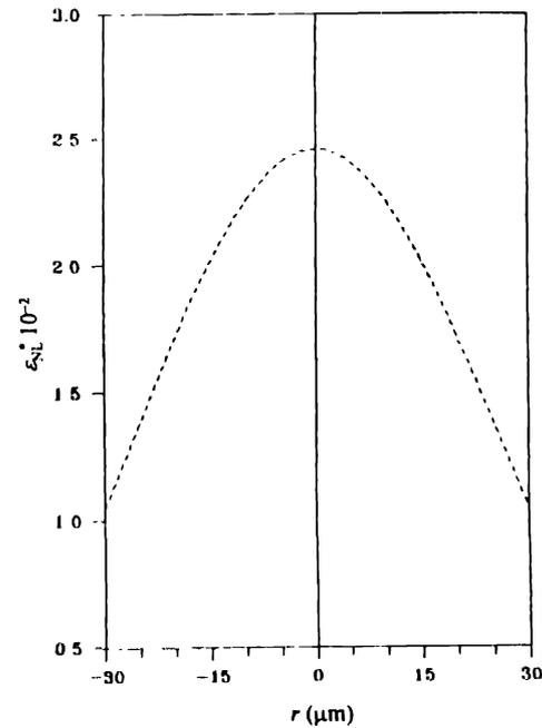
Figure 1. Radial profile of nonlinear part of dielectric constant ( $\epsilon_{NL}$ ) of plasma for ponderomotive nonlinearity. Here  $r_0 = 30 \mu\text{m}$ ,  $\beta E_0^2 = 0.55$ ,  $\omega_p = 2.5 \times 10^{13}$  rad/sec and  $\omega = 1 \times 10^{14}$  rad/sec.
