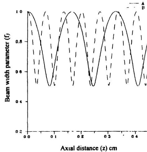
Figure 3. Oscillatory behaviour of self focusing beam width parameter ( $f$ ) with axial distance ( $z$ ) for ponderomotive nonlinearity. Curve (A) for present entire spatial beam analysis (non paraxial) and curve (B) for paraxial method  $\omega_p = 2.5 \times 10^{13}$  rad/sec,  $\omega = 1 \times 10^{14}$  rad/sec,  $\beta E_0^2 = 0.55$  and  $r_0 = 30 \mu\text{m}$
