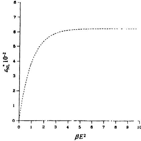
Figure 2. Nonlinear part of dielectric constant ( $\epsilon_{NL}$ ) variation with the beam intensity parameter ( $\beta E_0^2$ ) for ponderomotive nonlinearity in plasma.  $\beta = \frac{3m\alpha}{4M}$
