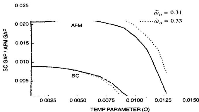
Figure 1. The plot of SC GAP ( $z$ ) / AFM GAP ( $h$ ) vs  $\theta$  for two different values of Debye frequency  $\tilde{\omega}_D = 0.31, 0.33$  for fixed value of  $\lambda_1 = 0.15$ ,  $\lambda_2 = 0.003$ .
