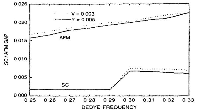
Figure 4. The plot of SC GAP ( $z$ ) / AFM GAP ( $h$ ) vs. Debye frequency ( $\tilde{\omega}_D$ ) for fixed values of  $\lambda_1 = 0.15$ ,  $\lambda_2 = 0.185$  and two values of  $V = 0.003$  and  $V = 0.005$ .
