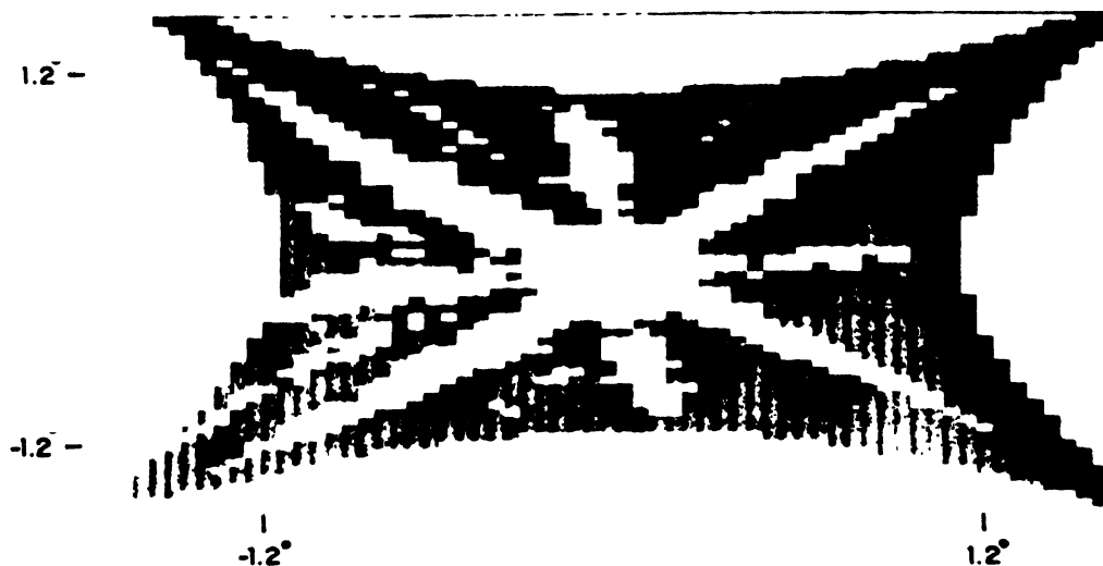
Figure 1. \langle 100 \rangle blocking pattern for elastically scattered ^{16}\text{O} (36 MeV) from Si crystal.
