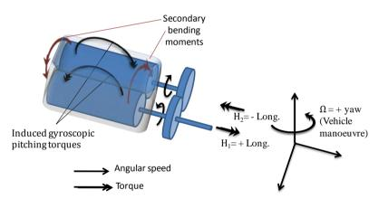
Figure 2.11 The figure shows the reaction torques for each flywheel, and the resulting bending moments on the flywheel package for a precession ( $\Omega$ ) yawing motion.
