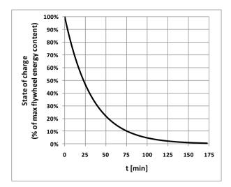
Figure 4.6 Flywheel state of charge with energy losses of 3% per minute.
