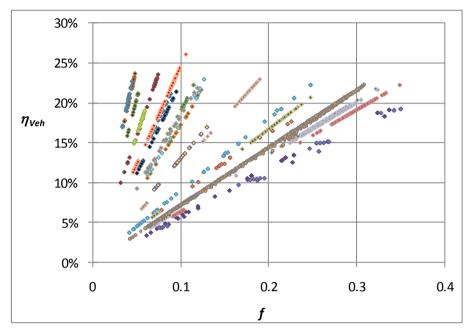
Figure 5.14 Plot showing the linear relationship between the factor defined in equation (5.3) and vehicle effectiveness. Each line corresponds to a different drive cycle, and the slope is the minimum average power required to drive the vehicle.
