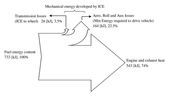
Figure 5.18 Energy flow through the *ideal-parallel-hybrid vehicle* from fuel to wheels, for the same conditions as the conventional vehicle presented in section 4.3, The contrast with Figure 5.1 and Figure 5.2 is quite interesting as it can be appreciated that the largest energy saving comes from a substantial decrease in fuel usage, which is possible by the powering of the vehicle through the reutilisation of the inertial energy of the vehicle.
