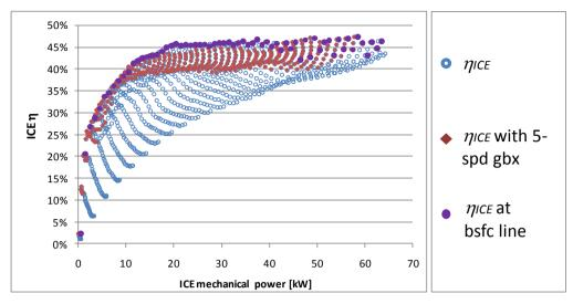
Figure 5.13 Thermal efficiency versus developed mechanical power for the ICE presented in Figure 4.3. The blue markers represent the possible operating area of the ICE, the red markers represent the area of operation when applying a shifting strategy with a 5-speed gearbox, and the purple markers represent the line of bsfc achievable with a CVT transmission.
