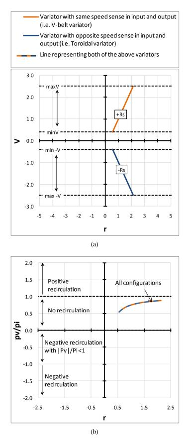
Figure 3.3 (a) Variator ratio as transmission ratio changes and (b) fraction of input power through the variator for six different configurations with different gear ratios  $G_V$ ,  $G_M$  and PGS size, providing the same power split and transmission ratios. The (+R) and (-R) labelled curves corresponds to a variator where the input and output angular speeds have the same sense and an opposite sense respectively.
