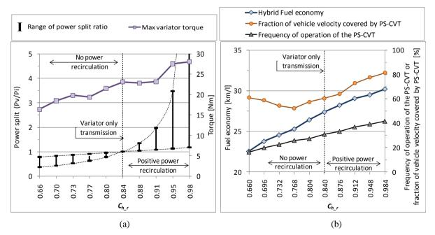
Figure 8.7 Simulations using the UDDS for a lossless transmission and flywheel. Plot (a) shows the range of power split (i.e. power through the variator) as the normalised ratio coverage is increased. Power split is less than one (i.e. no power recirculation) when the ratio coverage of the transmission is less than that of the variator, and conversely it is greater than one when it is greater. The maximum torque through the variator is also shown.
