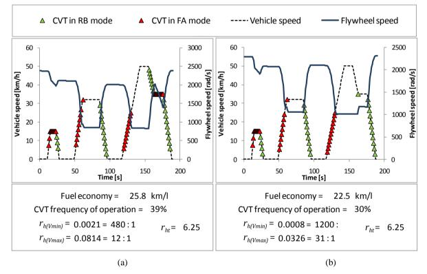
Figure 6.11 Plots (a) and (b) show the operation of the variator transmission in series with a two-speed gearbox for two different minimum *hybrid transmission ratios*. Plot (a) shows that a careful choice of gear ratios  $G_{hyb}$  and  $G_{fw}$  (which determine this minimum ratio) results in a system that is able to operate over a wide range of vehicle speeds. Further decreasing the transmission ratio greatly limits the use of the system at higher speeds as seen in plot (b).
