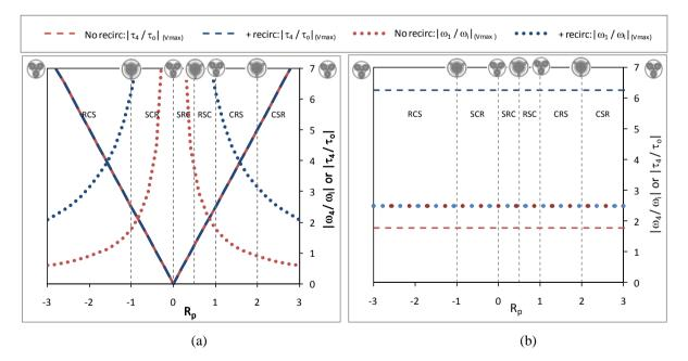
Figure 3.5 Maximum and minimum ratios of torque through the variator to output torque as  $R_p$  and PS-CVT configurations change for Case I (a) and Case II (b). The figures also show the ratio of variator speed to output speed for those conditions. The relative size of the sun to ring gears is also shown at the transition lines between the PS-CVT configurations for reference.
