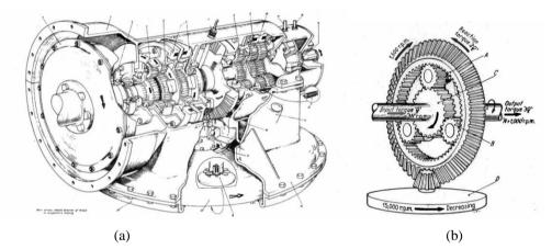
Figure 2.1 (a) The *Gyreacta* transmission developed for a bus application. (b) An example on the operation of the planetary gear set during an acceleration event.
