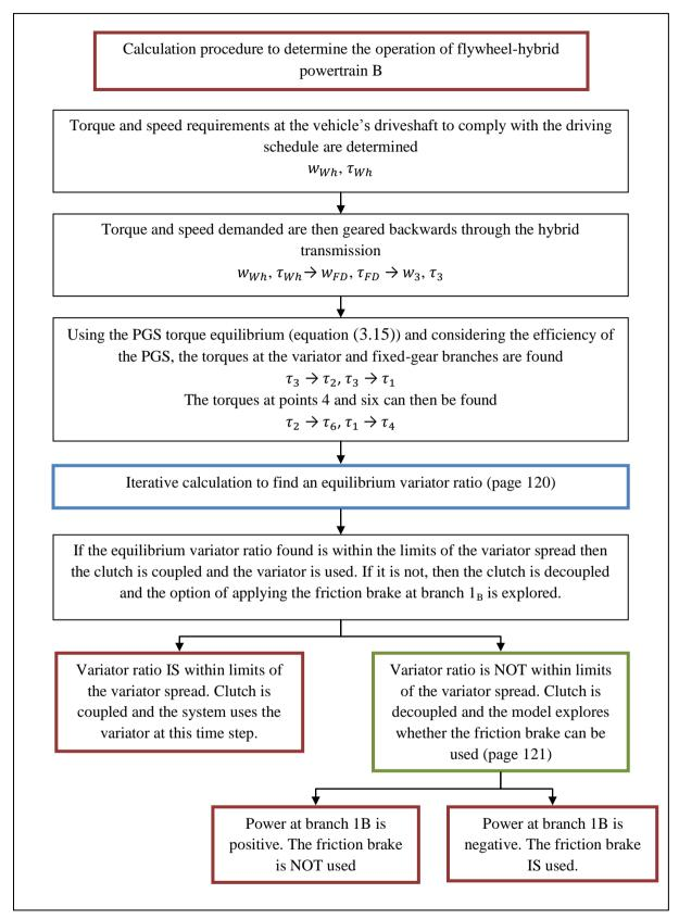
Figure 4.10 Flow diagram of the calculation procedure for the operation of *flywheel-hybrid powertrain* B. The procedure for other powertrains is similar.
