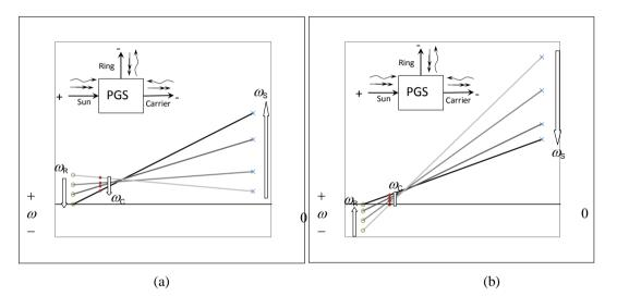
Figure 8.2 Nomogram showing (a) a regenerative braking event and (b) an acceleration event using a flywheel. The speed, torque and power senses for both conditions are also shown.
