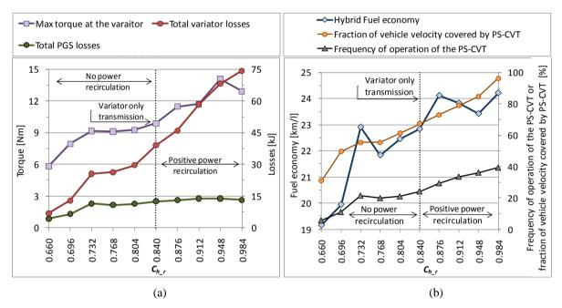
Figure 6.7 Plot (a) shows the losses of the variator unit and the PGS as the ratio coverage and power split of the transmission increases, showing a detrimental effect on fuel economy. The maximum torque through the variator is also shown,
