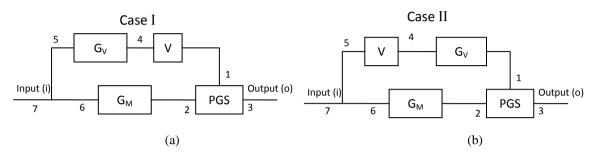
Figure 3.4 IC transmissions with (a)  $G_V$  at the input side of the variator, and (b)  $G_V$  at the output side of the variator.
