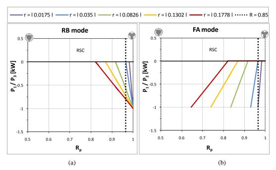
Figure 3.7 Ratio of power at the brake to PGS input power against planetary ratio  $R_p$  for different transmission ratios r at (a) RB mode  $(P_1/P_3)$ , and (b) FA mode  $(P_1/P_2)$ . The dotted line corresponds to a PGS with  $R_p = 0.965$  as the one used in [50].
