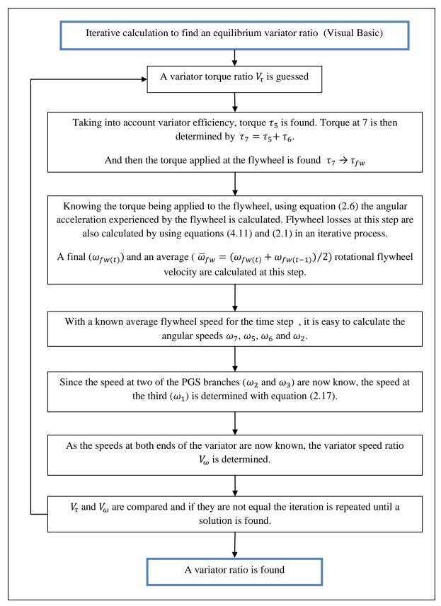
Figure 4.11 Flow diagram for the iterative calculation to determine an equilibrium variator ratio. This calculation s performed in Visual Basic.
