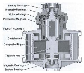
Figure 2.4. Cross section of the flywheel used by the University of Texas in hybrid bus.
