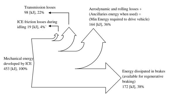
Figure 5.1 Final destination of the mechanical energy developed by the internal combustion engine for a vehicle following an urban drive cycle (Ford Focus Estate following the UDC cycle).
