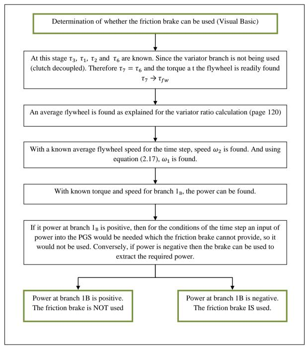
Figure 4.12 Flow diagram for the calculation that determines whether the friction brake can be used. This calculation s performed in Visual Basic.
