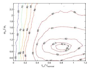
Figure 4.8 Efficiency map for the variator, adapted from Soltic [90].
