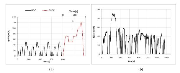
Figure 4.2. (a) the Urban (UDC) and Extra Urban (EUDC) Drive Cycles, and (b) the US Urban Dynamometer Driving Schedule (UDDS).
