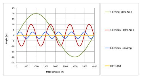
Figure 5.3 Examples of the road topology employed for the Sinusoidal gradients study-set.
