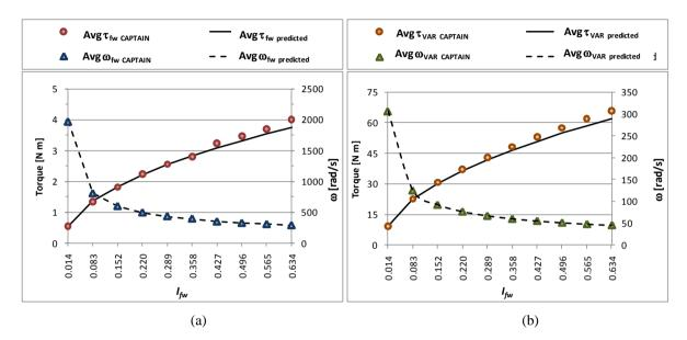
Figure 6.5 Taking into account the efficiencies and weights of the components, plot (a) shows the average torques and angular speeds achieved by the flywheel in the simulations as the inertia of the flywheel changes with predicted values shown as well. Plot (b) shows the corresponding average torque and angular speed of the variator along with their predicted values.
