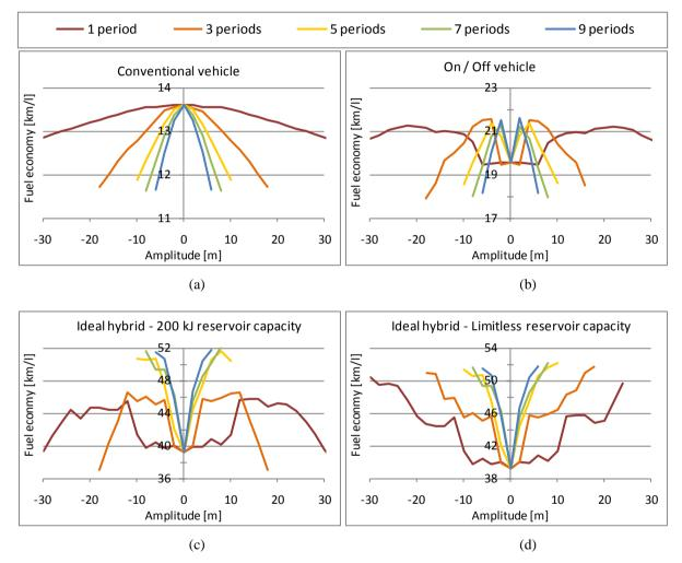
Figure 5.8 (a) The fuel economy of the *conventional vehicle* (b), the *ON/OFF vehicle* (b), the *ideal-parallel-hybrid vehicle* with a 200 kJ energy reservoir capacity (c), and the hybrid powertrain with a limitless energy reservoir capacity.
