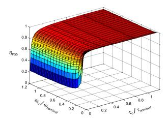
Figure 4.7 Efficiency map used to estimate the efficiency of the PGS. The map was normalised from an existing map in ADVISOR for the first gear of a Volkswagen 5-gear transmission.
