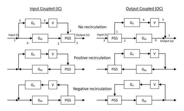
Figure 3.1 Operating modes for the Input Coupled and Output Coupled transmissions during FA mode.  $G_V$  and  $G_M$  are fixed gears of the variator and fixed ratio branches respectively. V is the variator unit and PGS is the planetary gear set.
