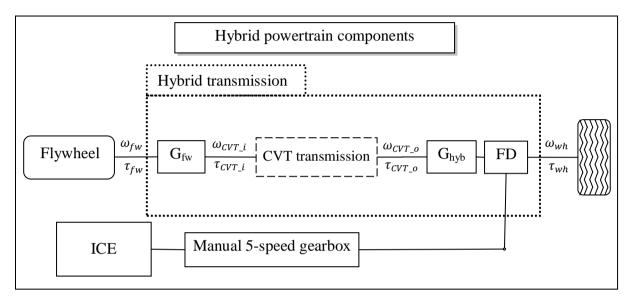
Figure 6.1 Schematic diagram showing the components common to all hybrid powertrains along with the relevant nomenclature.
