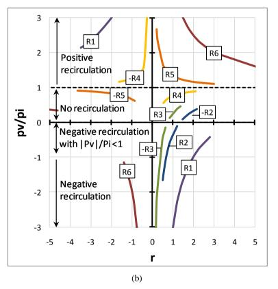
Figure 3.2 (a) Variator ratio as transmission ratio changes and (b) fraction of input power through the variator for six different PGS configurations with equal gear ratios  $G_V$ ,  $G_M$  and PGS size. Only the possible operation areas attainable through the variator range are shown.
