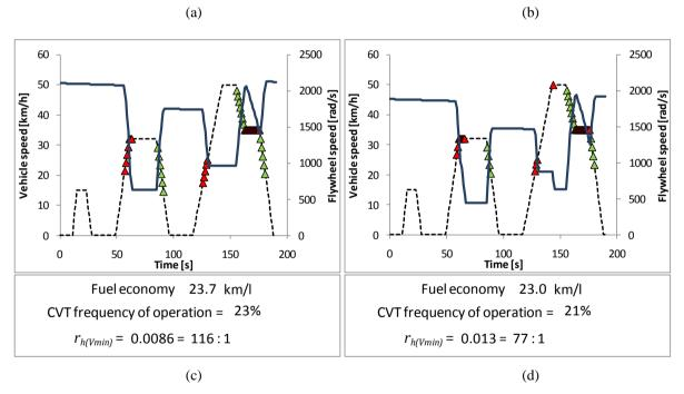
Figure 6.10 Plots (as) through (d) show the operation of the variator-only transmission with no gearbox for different minimum *hybrid transmission ratios*. The transmission spread is the same for all transmissions, but the minimum and maximum ratios which can be adjusted by varying  $G_{hyb}$  and  $G_{fw}$ , cause the hybrid system to operate at different vehicle speeds. The limited ratio coverage of the transmission makes it highly sensitive to the choice of fixed gears and drive cycle.
