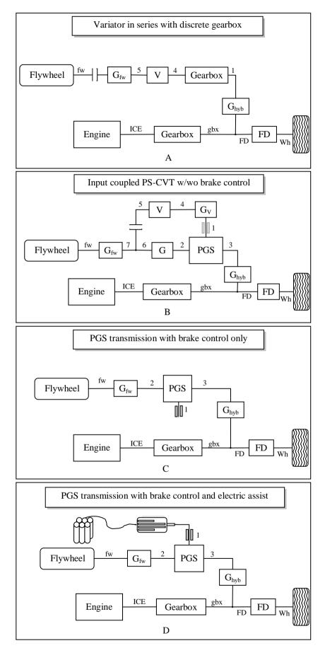
Figure 4.5 Schematic representation of the flywheel-hybrid powertrains simulated in CAPTAIN.
