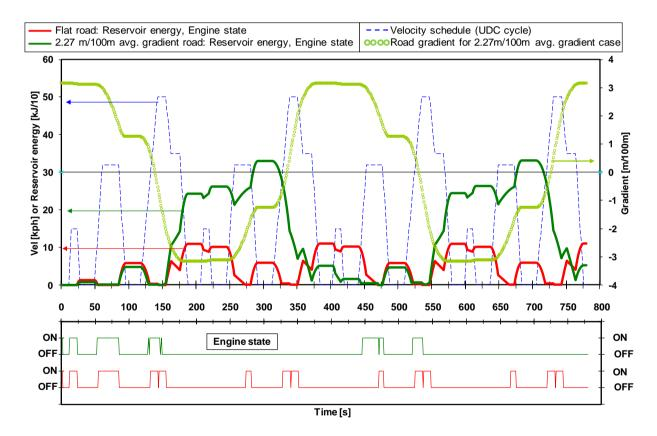
Figure 5.11 Operation of two simulations with different gradients: one on a flat road and one with 2.27 m / 100 m average gradient for the *ideal-parallel-hybrid vehicle* with a limitless energy reservoir capacity. The top chart shows the energy contained in the energy reservoir for each of the cases, as well as the gradient curve over time of the second case, and the driving cycle (UDC). The bottom chart shows the engine state (ON or OFF).
