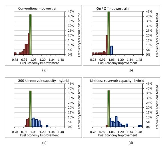
Figure 8.6 Frequency distribution plots of fuel economy improvement (measured as the improvement in fuel economy for each case over its performance in a flat road) for all gradients tested for the *Real Gradients* study-set. The red green and blue columns represent the frequency of cases exhibiting a worse, equal (or insignificant) or better fuel economy than the zero-gradients case respectively.
