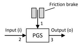
Figure 3.6 Transmission with a planetary gear set and a friction brake as control device in FA mode. During RB mode the input becomes branch 3 and the output branch 2.
