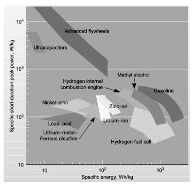
Figure 1.7. Ragone plot of energy storage technologies, showing their power and energy densities. Source: Science & Technology Review [25]
