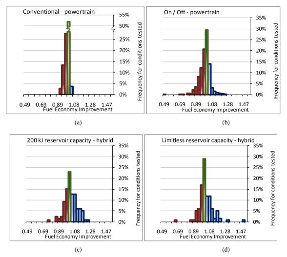
Figure 5.12 Frequency distribution plots of fuel economy improvement (measured as the improvement in fuel economy for each case over its performance in a flat road) for all gradients tested for the *Random Gradients* study-set. The red green and blue columns represent the frequency of cases exhibiting a worse, equal (or insignificant) or better fuel economy than the zero-gradients case respectively.
