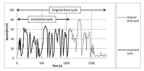
Figure 5.6 A Vancouver drive cycle with the original full drive cycle and the section used in the simulations.
