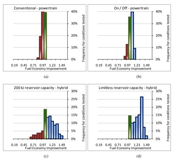
Figure 8.5 Frequency distribution plots of fuel economy improvement (measured as the improvement in fuel economy for each case over its performance in a flat road) for all gradients tested for the *Sinusoidal Gradients* study-set. The red green and blue columns represent the frequency of cases exhibiting a worse, equal (or insignificant) or better fuel economy than the zero-gradients case respectively.
