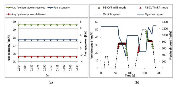
Figure 6.2 Plot (a) shows the fuel economy achieved by the hybrid vehicle for all flywheel inertias for a lossless hybrid transmission. Average power received and delivered by the vehicle also remains constant. Plot (b) shows the first 200 seconds of the UDC cycle for the simulation with inertia  $I_{fw} = 0.083$ . This plot illustrates the operation of the PS-CVT transmission and is the same for all the inertias investigated.
