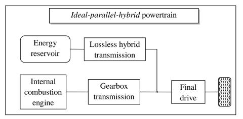
Figure 4.4. Schematic representation of the Ideal-parallel-hybrid powertrain
