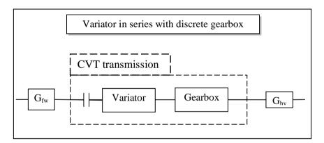
Figure 6.9 Schematic diagram of a CVT transmission consisting of a variator and a two-speed gearbox. In this transmission, the maximum and minimum *hybrid transmission ratios* attainable, which occur at the speed-ratio limits of the variator  $V_{max}$  and  $V_{min}$  are given respectively by
