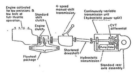
Figure 2.2. Schematic diagram of the series hybrid powertrain proposed by the Wisconsin group.
