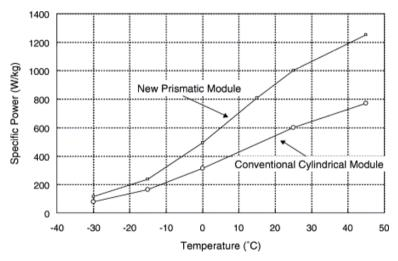
Figure 2.7 Power dependence of a Panasonic NiMH batteries on temperature at 60% SOC [53].
