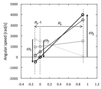
Figure 2.13 Nomogram for the kinematic equilibrium of a PGS with an  $R_4$ =0.9. The figure illustrates the equilibrium speeds during a regenerative braking event. It can be seen that as the ring and carrier (vehicle) decelerate, the sun (flywheel) accelerates, maintaining the linear kinematic relationship as defined in equation (2.17).
