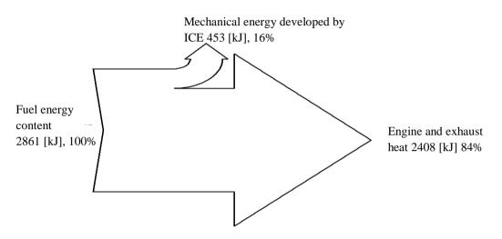
Figure 5.2 Thermal efficiency of the ICE following the UDC cycle.
