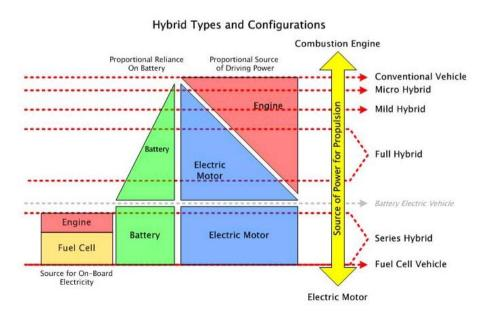
Figure 2.6. Hybrid types according to their use of batteries and their source of driving power. Source: Green Energy Congress [51]
