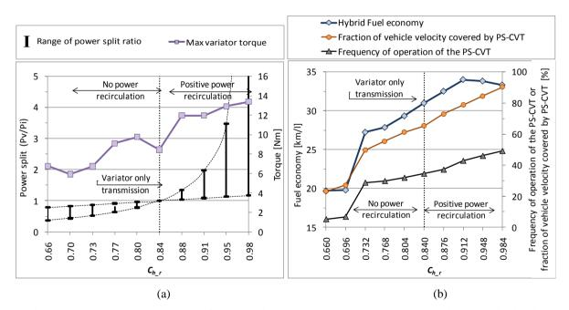
Figure 6.6 Plot (a) shows the range of power split (i.e. power through the variator) as the normalised ratio coverage is increased. Power split is less than one (i.e. no power recirculation) when the ratio coverage of the transmission is less than that of the variator, and conversely it is greater than one when it is greater. The maximum torque through the variator is also shown.
