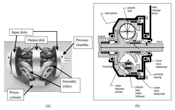
Figure 2.15 (a) Parts of a Torotrak toroidal variator [83], (b) a Milner rolling variator [82].
