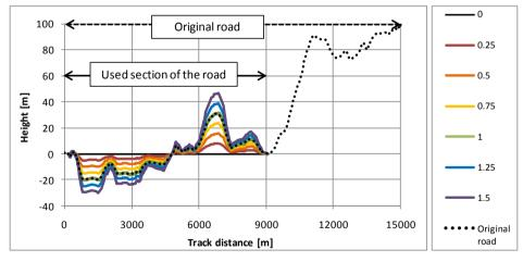
Figure 5.7 The corresponding topology for the drive cycle shown above, showing the section used of the road along with the different fractions of road gradients magnitudes used.
