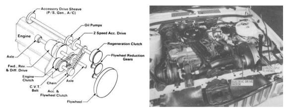
Figure 2.3 Transmission and installation of the flywheel used by the General Motors group.
