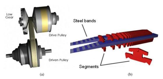
Figure 2.14 (a) A V-belt variator in low gear, (b) elements of the transmission belt. Figures taken from [76].
