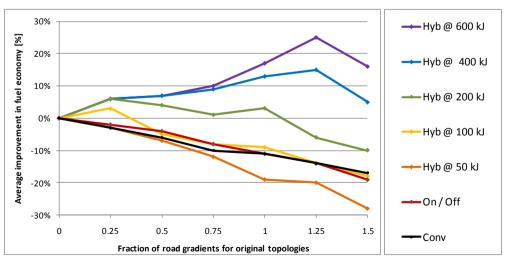
Figure 5.10 Average fuel economy improvement (compared to the base case of a road with zero-gradients) as the magnitude of road gradients in increased, for various vehicle and with different energy reservoir capacity limits. In the graph, a fraction of road gradients of zero corresponds to a flat road, and a magnitude of one corresponds to the original topology of the road.
