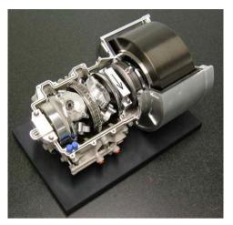
Figure 2.5 Flybrid Formula One Kinetic Energy Recovery System. Source: www.flybridsystems.com
