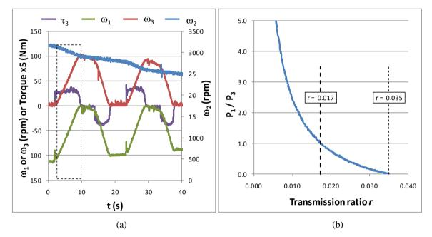
Figure 3.8 (a) An experimental run for FA mode and (b) the transmission ratio versus ratio of power at the brake to power at the output  $(P_1/P_3)$  for the boxed area in plot (a).
