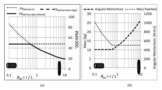
Figure 2.10. Plot (a) on the left shows the dependency of  $\omega_{max}$  changes from the  $\omega_{max}$  allowed by the bearings to the  $\omega_{max}$  allowed by the maximum tensile stress of the material as the ratio R increases. Plot (b) shows the effect that these dependencies have on the mass and angular momentum of the flywheel.
