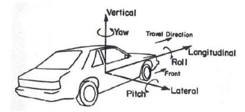
Figure 2.9 Vehicle axis system and vehicle manoeuvres used to describe gyroscopic motion [69].
