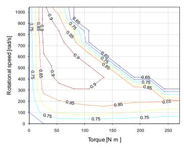
Figure 8.3 Efficiency map for a 75 kW AC Induction motor.
