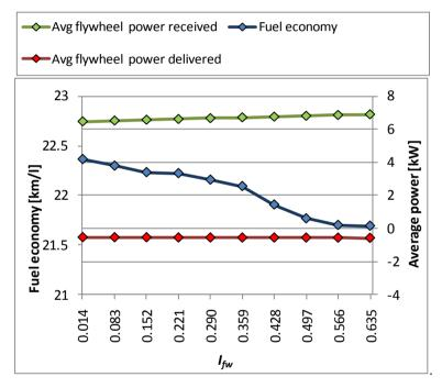
Figure 6.4 Shows the fuel economy achieved by the hybrid vehicle for all flywheel inertias when considering the efficiencies and weight of the components. Average power received and delivered by the vehicle remains fairly constant.
