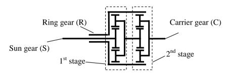
Figure 8.1 A double stage planetary gear set (PGS).
