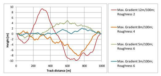
Figure 5.5 Two examples of randomly generated road topologies with varying maximum gradients and road roughness.
