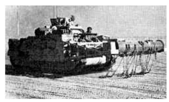
Figure 4. The Matilda-Scorpion Flail Tank. The Flails were designed to detonate the mines in order to create a clear passage through a mine field.
