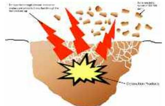
Figure 1d. The detonation products are vented through the voids in the soil resulting in the ejection of soil.
