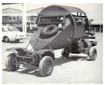
Figure 6. The Leopard. It incorporated the V-shaped hull with the single monocoque hull which provided protection to the drive-train as well as the passenger compartment. The increased axle length brought the wheels outside the passenger compartment and the easily sheared connection meant that the wheel assembly would be blown clear of the vehicle if it detonated a mine. (Source: Ernest Konschel. Available from: http://www.baragwanath.co.za/leopard/)
