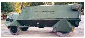
Figure 5. The Swedish SKPF M/42 Armoured Personnel Carrier developed during WW2 was the first vehicle to incorporate the V-shaped hull to aid deflection of the detonation products. This feature was later included in both Rhodesian mine vehicles and in modern coalition mine-protected vehicles.
