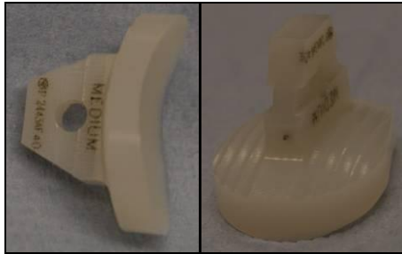
Figure 6.2: TOKL smooth keeled design with macrostructures. Note: Only large sized implants were tested.
