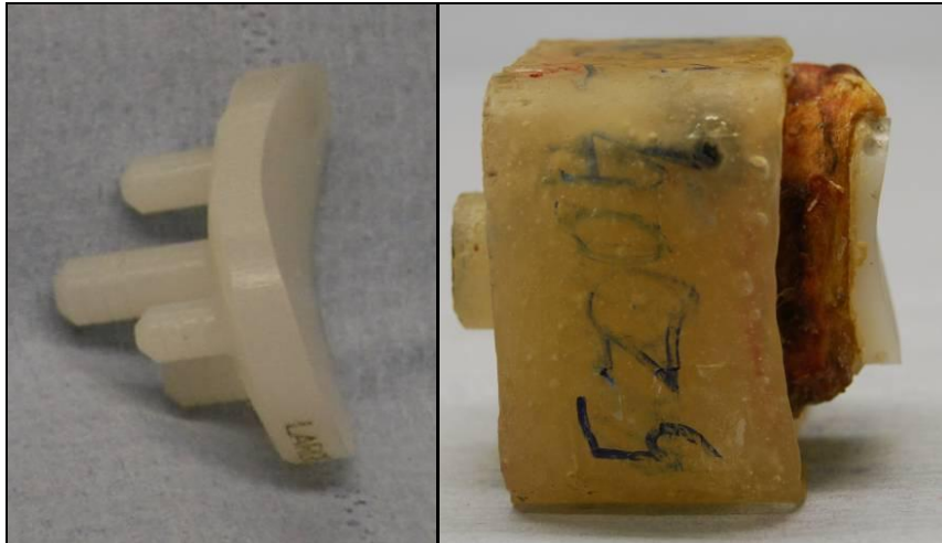
Figure 5.1: Aequalis Tornier curved-back cemented glenoid implant (left). NB2 specimen cemented and potted for testing (right).
