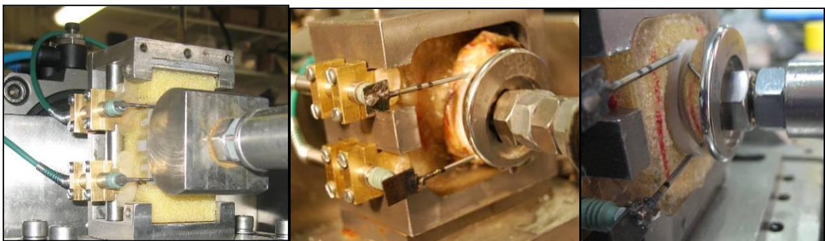
Figure 7.1: superiorly and inferiorly aligned LVDTs for rim displacement measures in 2D (left), cadaveric (middle) and 3D (right) studies. Note: figures are the same as Fig. 4.3, 5.2 and 6.4 respectively.
