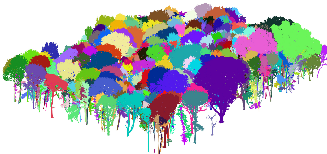
Figure 3. Segmented one hectare point cloud of Wytham Woods: 559 individual trees were extracted.
