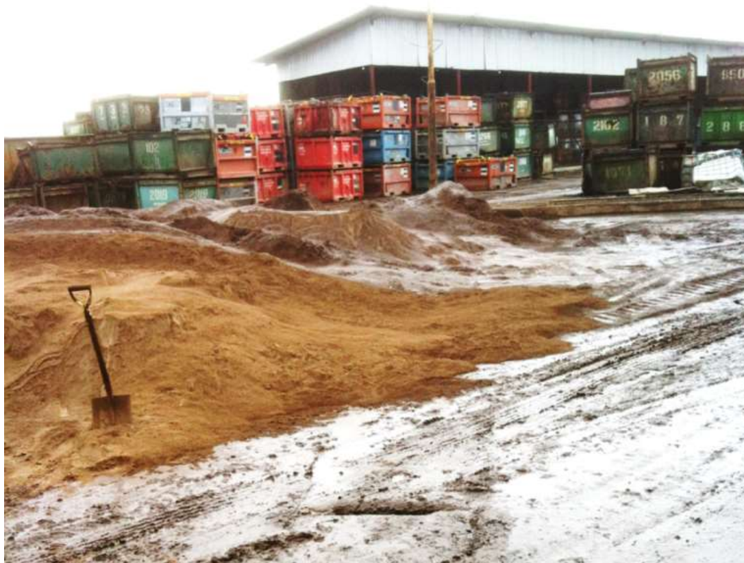
Figure 4. Heap of pre-treated drill cuttings from the anaerobic thermal desorption unit (ATDU) of a commercial treatment facility in the Niger Delta, Nigeria. Source: Corresponding Author.
