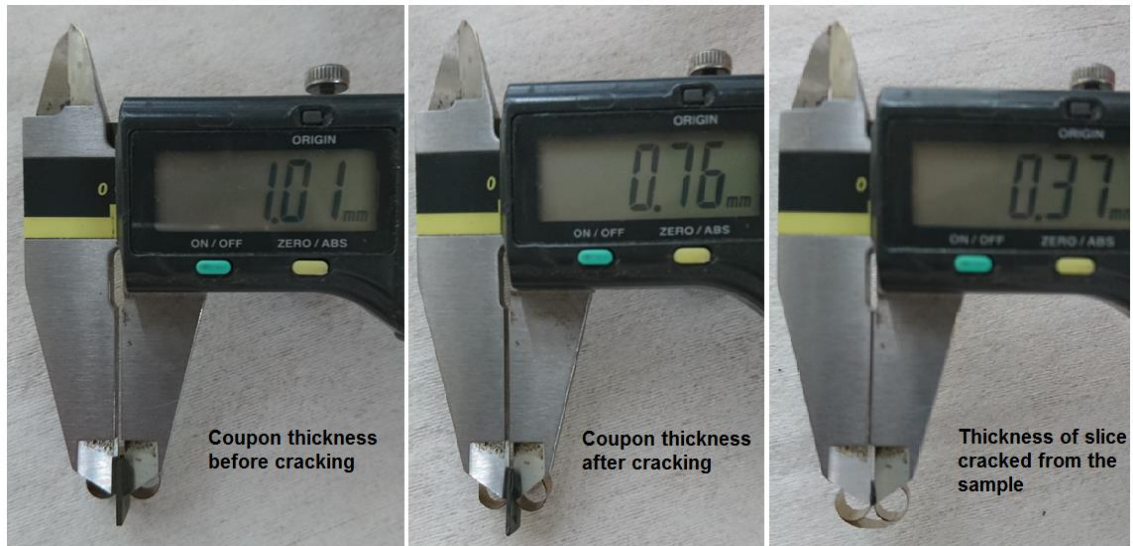
Figure 5. 5: Thickness values of the Ti-base alloy before cracking (left), after cracking (middle) and of a broken slice (right), pretreated at 1173 K
