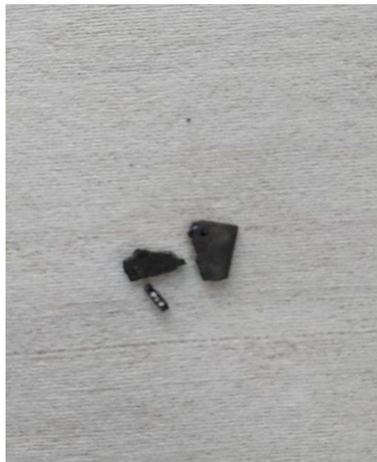
Figure 5. 6: Broken Ti-base alloy coupon after cracking pretreated at 1273 K
