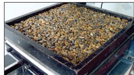
Figure 4. PUR mixed crushed stones.
