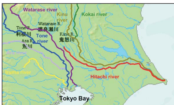
Figure 1. Eastward diversion of Tone river (modified from [2]): original course (left) and diverted course (right).
