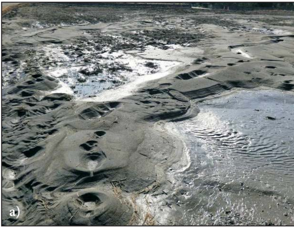
Figure 12. Extensive sand boiling (a) at the rice field in Toride city and (b) between residential houses in Abiko city.
