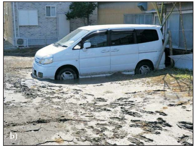
Figure 12. Extensive sand boiling (a) at the rice field in Toride city and (b) between residential houses in Abiko city.
