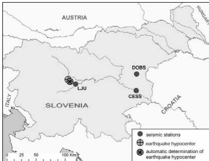
Figure 7. The map showing the locations of the seismic stations that contributed their data to the automatic determination of the earthquake's parameters, the hypocenter of the earthquake and the automatic determination of the hypocenter's location. Even with this small number of seismic stations, the automatic location is still close to the real one.
