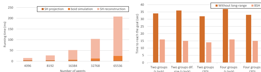
Fig. 2. Per-kernel runtime for the two-group z-lock scenario (left) and simulation runtime time for five tested scenarios (right).
