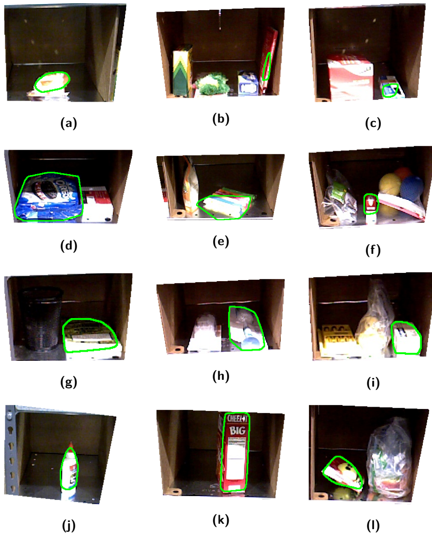
Figure 3.5: Segmentation results during the APC run; the green line outlines the segments returned by our method; all segments lie on the correct objects; mean precision: 91%, mean recall: 73%, F_{0.5} score: 0.864 (©2016 IEEE)
