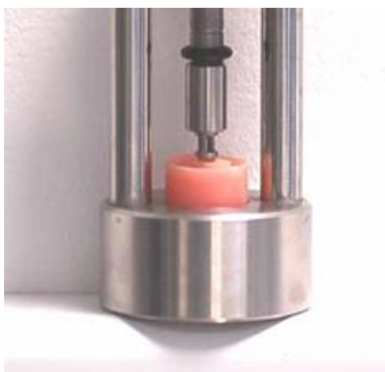
Figure 9.1. Cylindrical stainless steel mould (3.35 mm diameter) placed in the centre of the lithium disilicate specimen and filled with resin composite material (Tetric EvoCeram, Ivoclar Vivadent AG, Schaan/Liechtenstein). The resin composite was light cured for 40 seconds.
