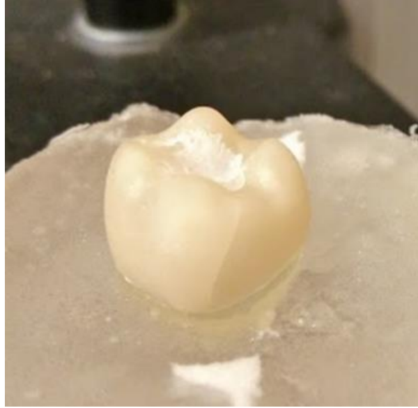
Figure 5.6 An example of a specimen after removal from storage in water at 37°C exhibiting a crack initiated at the distal buccal margin of the LDGC crown and propagated toward the distal cusp on the occlusal surface.
