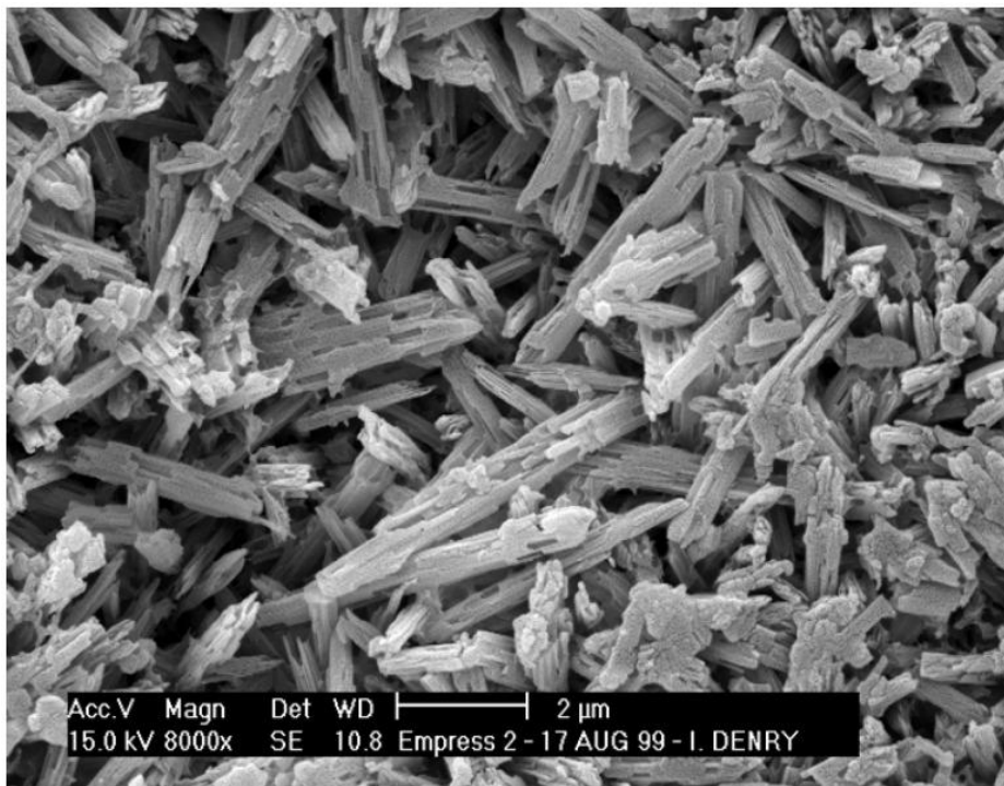
Figure 2.8 SEM image of lithium disilicate glass-ceramic, the lithium disilicate phase exhibits a rod-like morphology, which forms an interlocking microstructure (Denry and Holloway, 2010).
