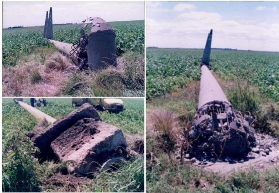
Figure 2: Damages of the pylons that support of electrical transmission network. (Courtesy of ENERSA S. A.)
