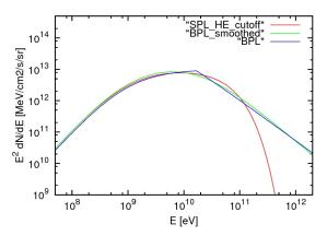
**Fig. 3.** Particle total energy distributions for our best hadronic models vs the kinetic energy: a simple power-law with a high-energy cut-off at  $E_c = 45 \text{ GeV}$  (Eq. 1, red), a smoothed broken power-law with  $E_{br} = 16 \text{ GeV}$  (Eq. 2, green), and broken power-law with  $E_{br} = 20 \text{ GeV}$  (Eq. 3, blue).
